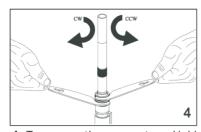
4. To remove the gas system. Hold the gas cylinder stationary with one wrench while turning the gas chamber lock nut in the direction indicated.
