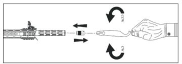
1) You must ensure that the choke is hand tight before firing.
