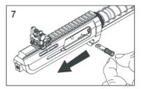
7. To lower the feed ramp you must hold the charging handle back while rotating the feed ramp lever to the downward
