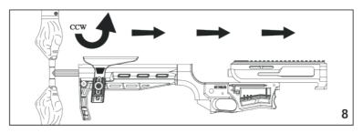
8. After removal of the butt stock bolt, you are now able to separate the upper receiver assembly from the lower receiver.
